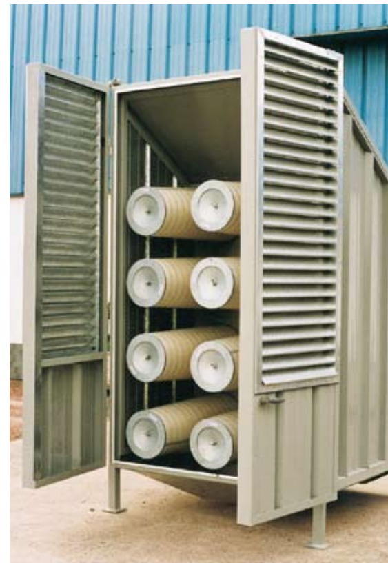
Filter module open for inspection.
